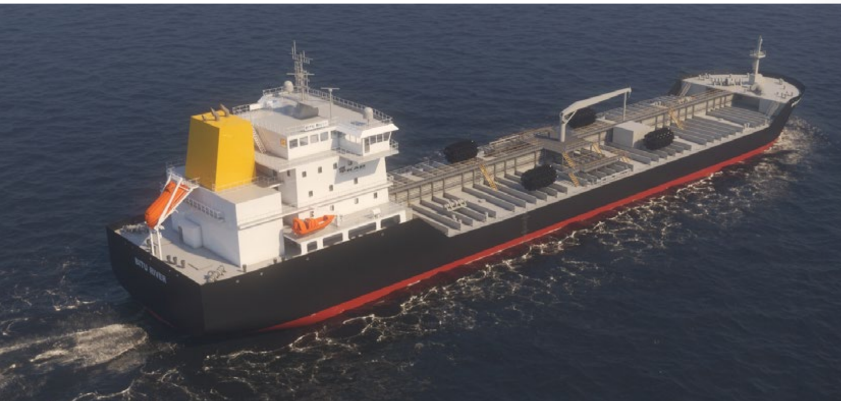
Picture: BITU RIVER, Bitumen Tanker, 14,500 dwt with twin azimuth thrusters and diesel-electric propulsion. Under construction in CMJL, Yangzhou, for Rubis Asphalt Middle East (RAME).
